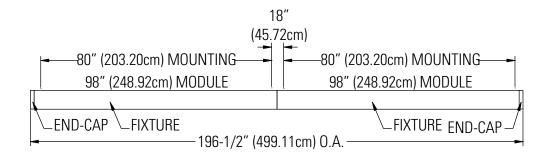
20' Continuous Run of Fixtures Type 3 (Three Modules in Run)
